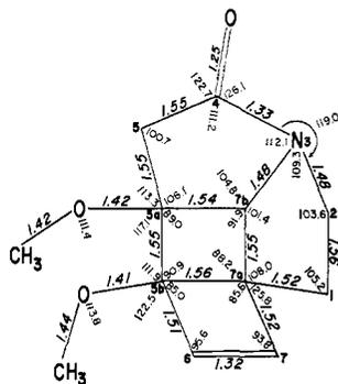
Figure 1. Bond distances and angles of compound V. Additional angles about atoms 5a, 5b, and 7a are as follows: 6-5b-5a,  $114.6^\circ$ ; O-5b-7a,  $126.0^\circ$ ; 5b-5a-5,  $116.1^\circ$ ; O-5a-7b,  $111.9^\circ$ ; 1-7a-5b,  $127.0^\circ$ ; 7-7a-7b,  $115.9^\circ$ .
